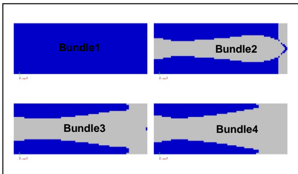
Level setting Ply-Bundles: 0° plies
