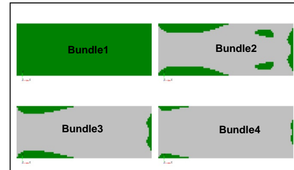
Level setting Ply-Bundles: 90° plies
