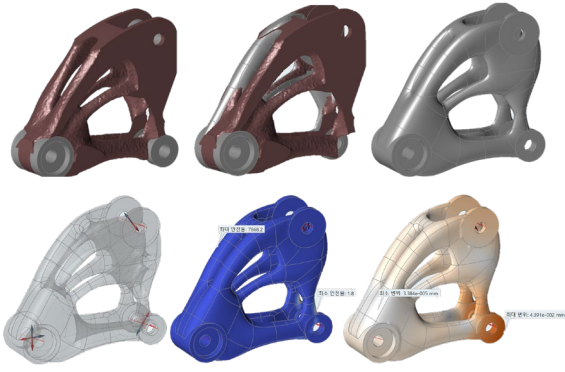
Fig. 8 PolyNURBS process and FEA results
