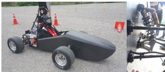
Fig. 14 Bell crank as installed on vehicle
