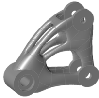
Fig. 9 3 rd optimization : gauge optimization result
