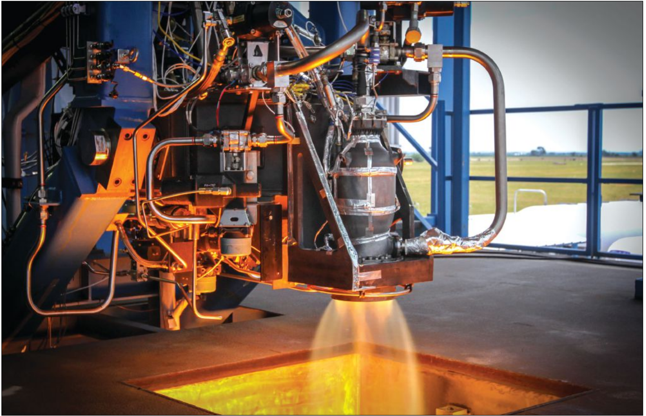
Rocket engine parts made by 3D manufacturing in copper alloy undergo hot-fire testing at NASA Glenn with Aerojet Rocketdyne.
